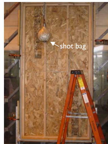
Fig. 3 – Photo showing impact of shot bag on wall's interior to create cracks in the scratch coat.
